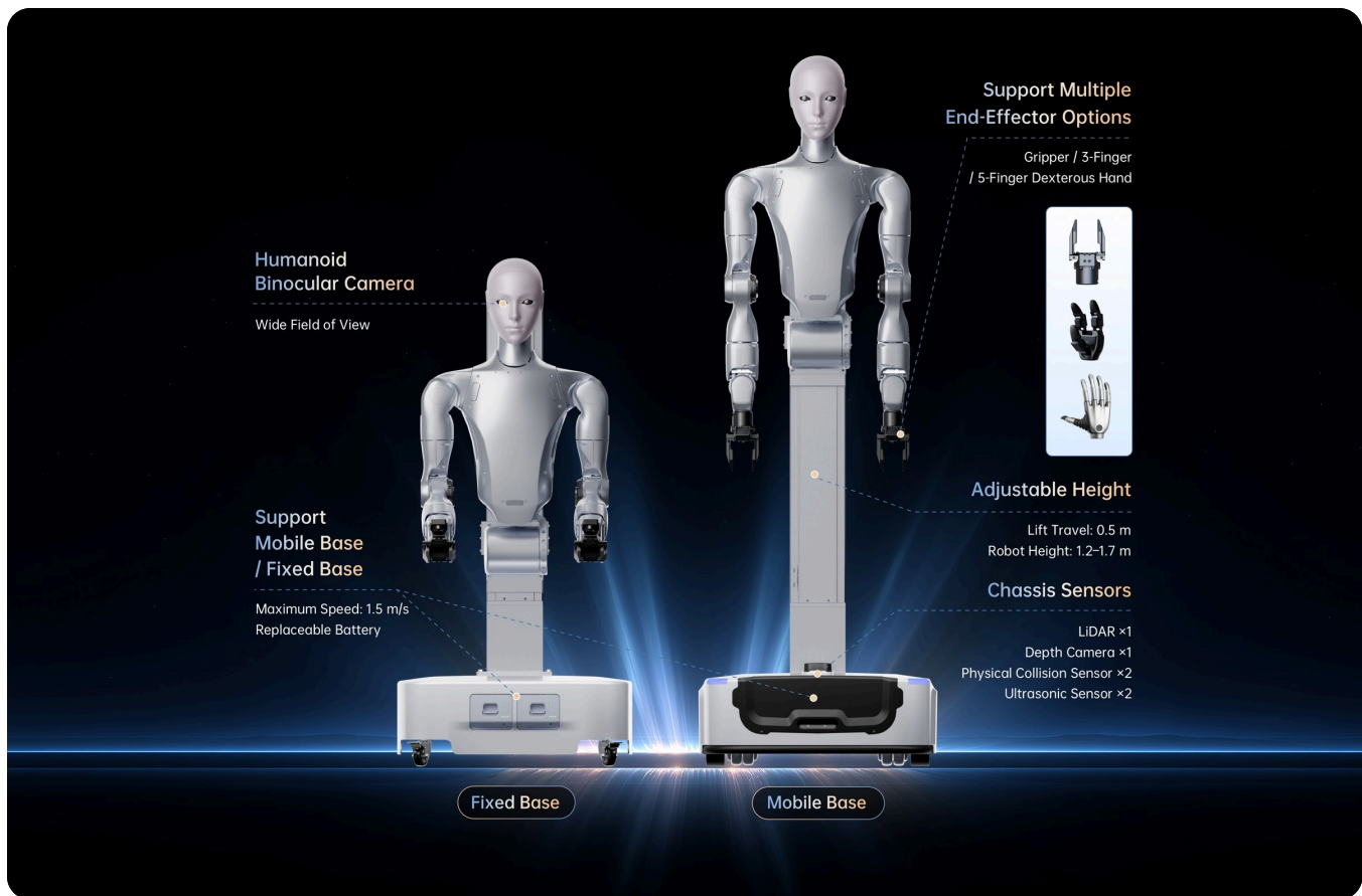
Unitree's H2-D callout graphic: the Standard on its fixed base (left) and the Flagship on its mobile base (right).
